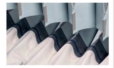
The connecting clips between bellows.
