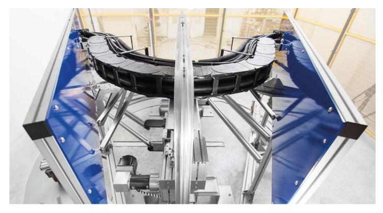
Internal complete hose guiding system with fixing brackets ready for assembly of all cables between carriages.
