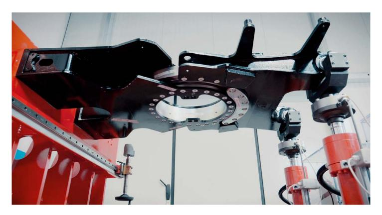
We can thus assess the strength and fatigue states of the materials and the reliability of the components over time.
